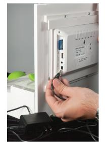
10. Plug power adapter into TV and power source.
